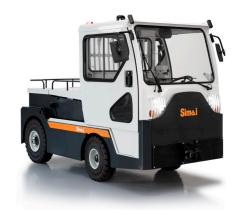
4-wheel tow tractor, man on board. Heavy-duty high-performance and long-range truck for industrial and airport handling duties. Despite its small size and turning radius, the TE252 has a high towing capacity and performances. Loading capacity of wide rear platform 200 kg.
